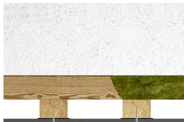
Horizontal batten with insulation slotted in. Vertical batten on the top with panel finish & screw
