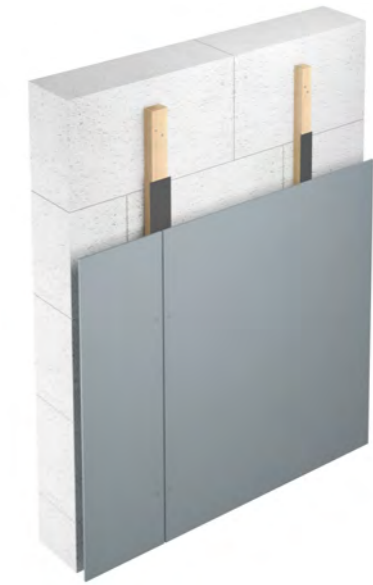
Construction with vertical battens
